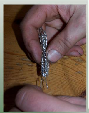
Use the mandrel to keep the core of the chain hollow and in approximately the right shape.
